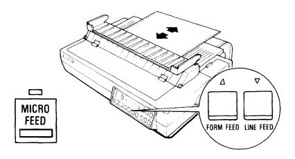
Note: The printer beeps when the paper reaches a position that is approximately 1/3 of an inch from the top edge of the paper. You can use this position as a reference point when you adjust the printer's loading position.
